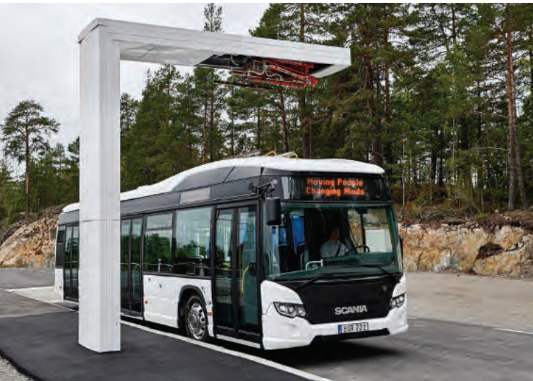
Figure 1: An Opportunity Charged Fully Electric Scania Bus and Pantograph
